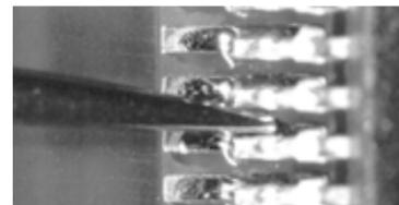
10 MilProbe straightening leads of 20 mil pitch QFP.
